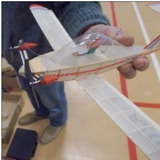
The motors for this twin were made as a matched pair
